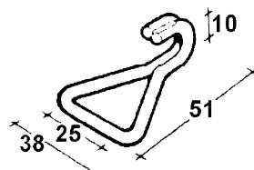
Breacking load 300 kg
